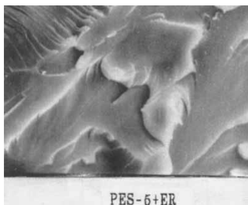
FIG. 8. Fracture surface of modified epoxy resin with PES.
